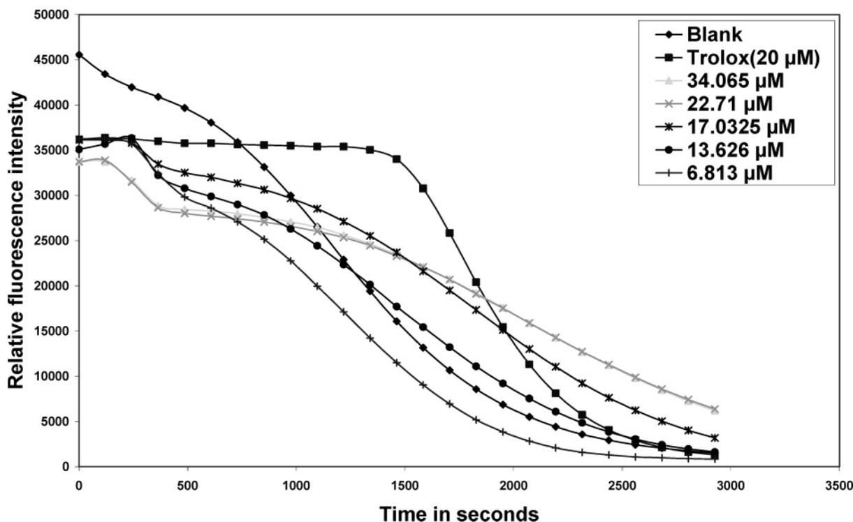
Figure 3. Fluorescence decay profiles induced by AAPH for lycopene at different concentrations in the presence of 0.4%  $\beta$ -cyclodextrin.
